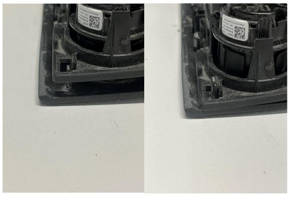
7. Now all you have to do is clip in the lower area. Attach the clips until some tension builds up and then help minimally with your fingers so that the clips can slide over the lower part. It also helps if you move the carbon front down a bit with your thumbs so that the frames snap into place better. Then reinstall the Torx screws and you can mount the part.
