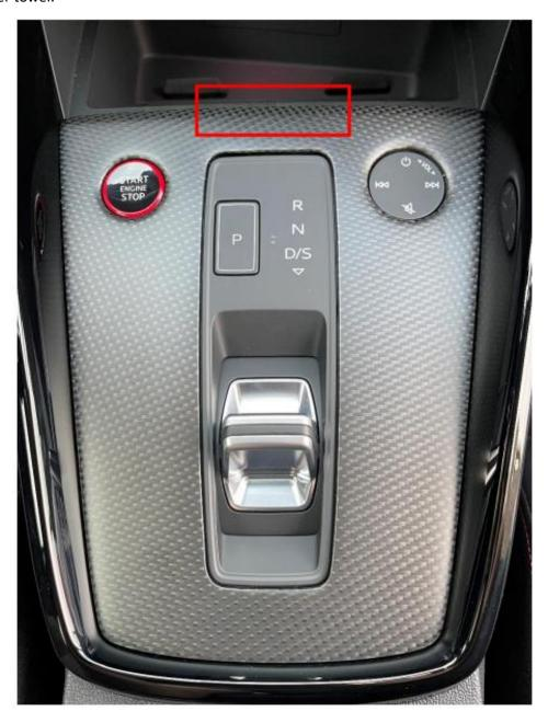
2. Remove the 4 plugs on the back. Gearbox connectors are squeeze and pull, media and start button have a latch (red) that must be unlocked. Then pull out. Take out the frame.
