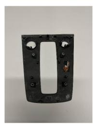
6. Put the back on. In the area of the media button, the parts have to be wobbled slightly past each other. Once the back is almost flush with the front, FIRST run the front back under the clip. Do not work with force here, the parts should be quite easy to slide into each other. It helps to lift the back area a bit when pushing together.
