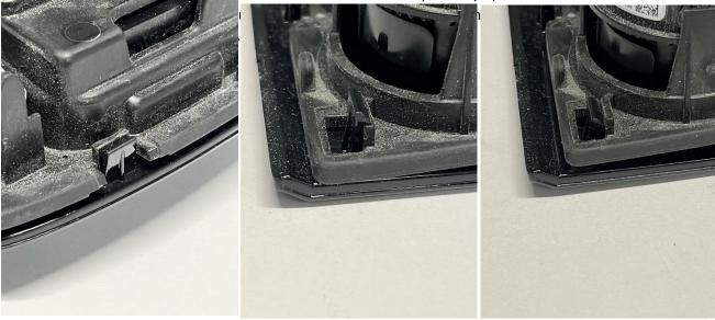
5. Remove the back by pulling upwards and transfer the knobs and selector levers to the new carbon part.
